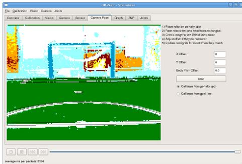
Figure 18: Off-Nao showing kinematic calibration of camera offsets.
