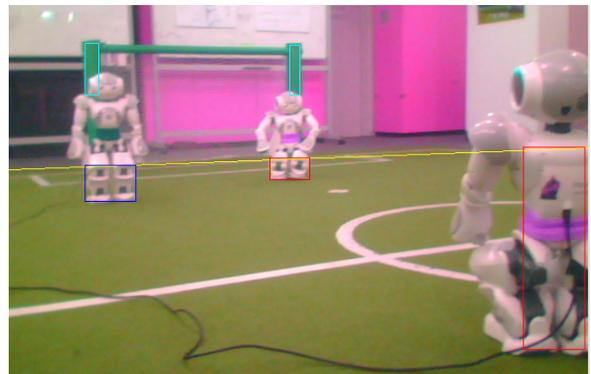
Figure 5: Detection of goal-posts, field-edge, and robots.
